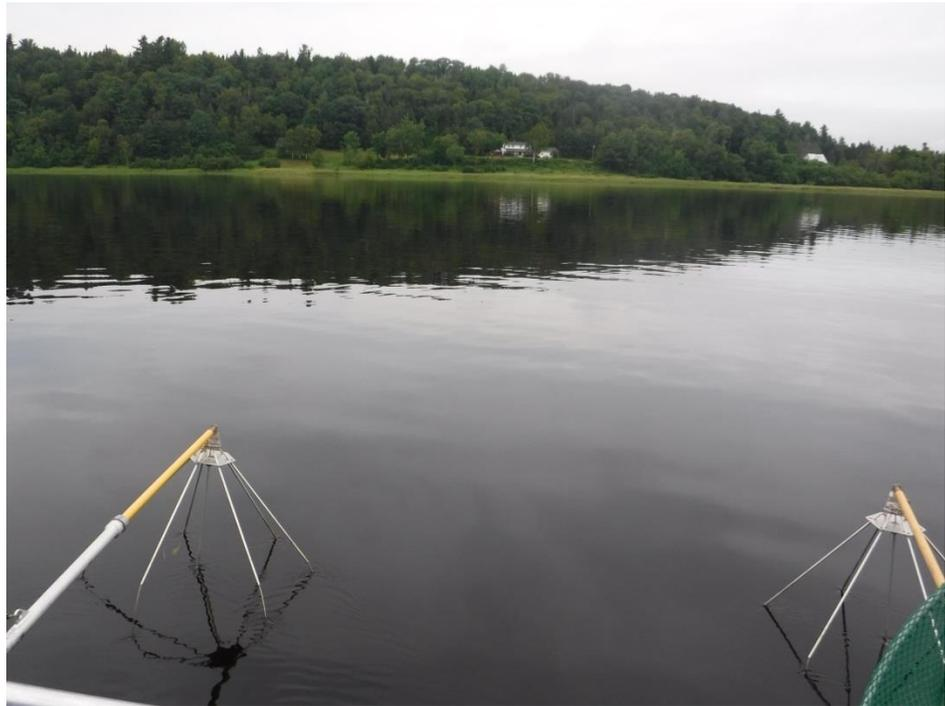
Above: The business end of the electro-fishing boat, the electrical current passes between the 2 electrodes. Two people stand on a platform in the front of the vessel to capture fish.
