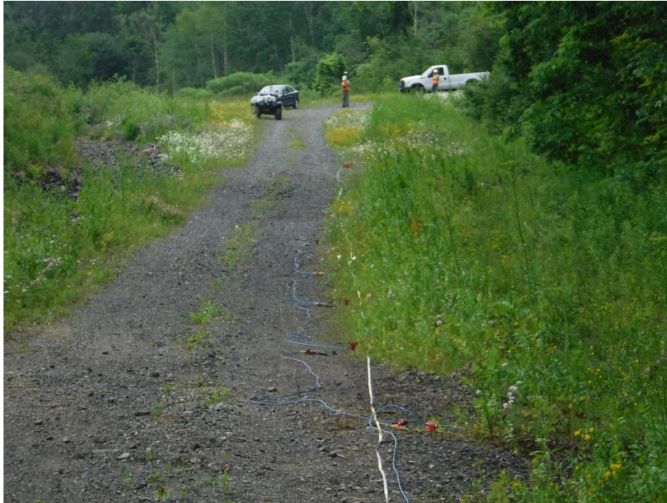
Above: Seismic sensor array with electrodes spaced at 5 meter intervals.
