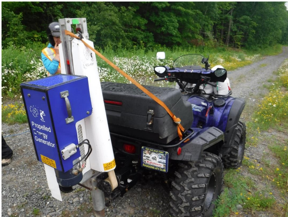
Above: Impact testing device (Propelled energy generator)
